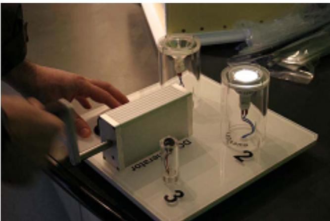
One answer is the use of energy efficient light bulbs, which you can then demonstrate using the light board. *Do they think the Halogen or LED is the energy efficient light bulb? Show the students how the generator works and get them all to light up both bulbs. What happens to the LED bulb? The faster the handle is turned, the brighter it is. Why? Which is the Energy Efficient bulb?*
