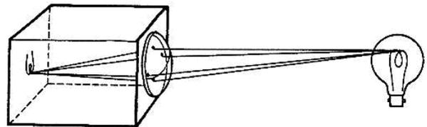
There are two different types of lens for the students to investigate. Ask them to try and image the lights on the ceiling onto the table (telling them to try and burn a hole in the table usually makes them realise what to do quickly) and observe how the focal length changes for the two different thickness lenses.
