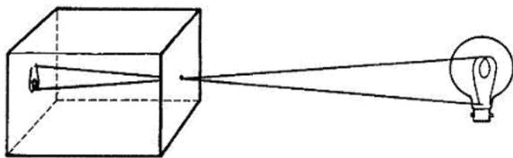
*The image is quite faint, how can we let more light in? Use the pin to create a larger hole and a few more holes. What happens? Can you work out which is the largest hole just by looking at the image? The brightest image is from the larger hole. But at what cost? The image has become blurred. More holes leads to multiple images. Again draw a quick diagram to explain.*
