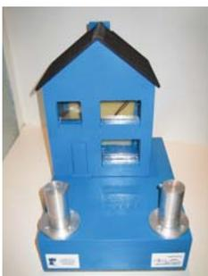
Sound (vibration) from the speaker causes the window to vibrate a very small amount. This movement interferes with the path of the laser. The change in path is picked up by the detector and then converted back into sound.
