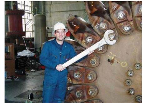
Full size Pelton wheel water turbine at an Hydroelectric powerstation.
